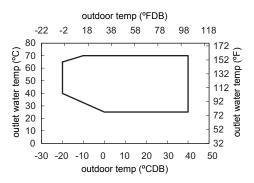
Outdoor temp -20°CDB/ Outlet water temp 40~65°C (Outdoor temp -4°FDB/ Outlet water temp 104°F~149°F) Outdoor temp -10°CDB/ Outlet water temp 33°C~70°C (Outdoor temp 14°FDB/ Outlet water temp 91°F~158°F) Outdoor temp 0°CDB/ Outlet water temp 25°C~70°C (Outdoor temp 32°FDB/ Outlet water temp 77°F~158°F)
