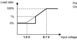
Preset temperature = 100% \* (Input voltage - 1.0) / 8.1 V Change of 59 mV or less is not recognized.
