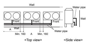
If the product width (labeled A in the figure) times the number of units that are installed side by side exceeds 6 m, leave a space of 1000 mm between each block. Each block is defined as a group of units that fit within 6 m.
