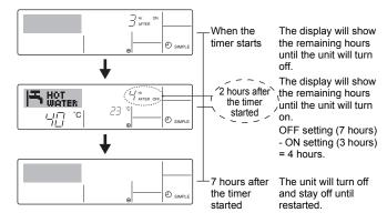
Example 2: The ON-timer is set to 5 hours, and the OFF-timer is set to 2 hours.
