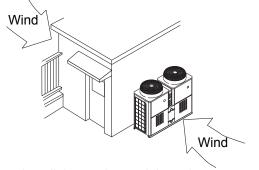
Install the outdoor unit in a place where it is not exposed to direct wind, such as behind a building.
