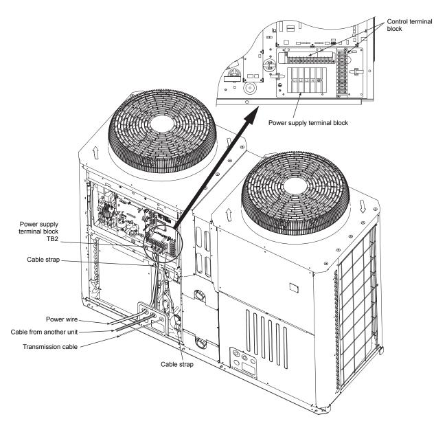
**Important:** Power supply cables larger than 25 mm<sup>2</sup> in diameter are not connectable to the power supply terminal block (TB2). Use a pull box to connect them.
