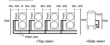
If the product depth (labeled B in the figure) times the number of units that are installed in rows exceeds 6 m, leave a space of 1000 mm between each block. Each block is defined as a group of units that fit within 6 m.
