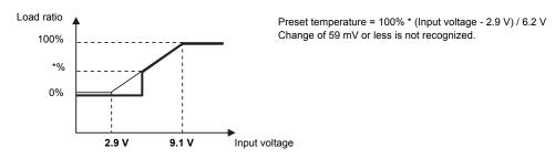
\*%: When the compressor frequency drops below 30 Hz, the compressor stops.
