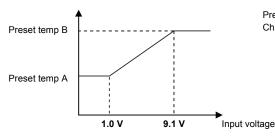
Preset temperature = (B - A) \* (Input voltage - 1.0 V) / 8.1 V + A Change of 59 mV or less is not recognized.
