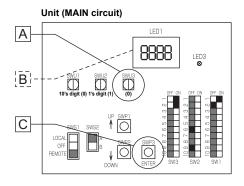
\*1 If the start-up process has already been completed, [FFFF] (instead of [EEEE]) will appear when the rotary switch SWU3 is set to "F."
