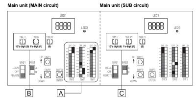
Make sure the address of the MAIN circuit on the main unit is set to "1" (labeled B in the figure above) and that the address of the SUB circuit on the main unit is set to "51" (labeled C in the figure above).
