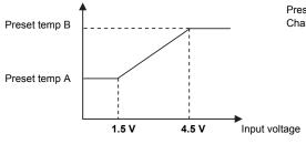
Preset temperature = (B - A) \* (Input voltage - 1.5 V) / 3.0 V + A Change of 29 mV or less is not recognized.
