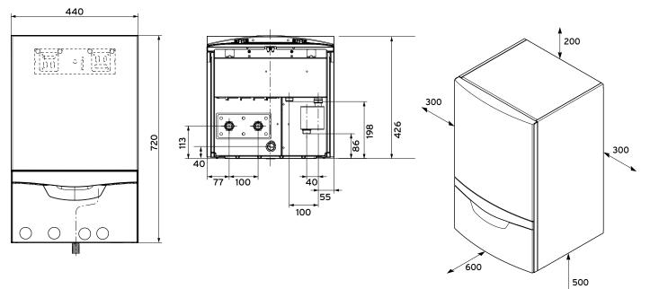
NOTE: all measurements are in mm
