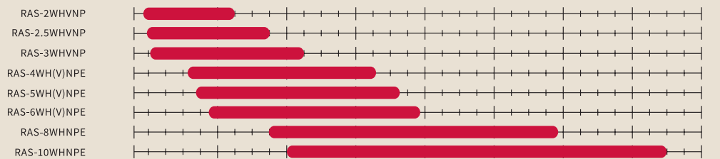
Heating capacity range under the conditions: water input/output: 30/35 °C; outside temperature: 7/6 °C (WB/DB).
